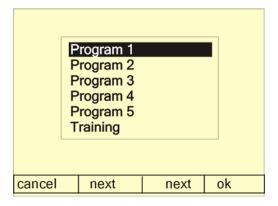
The exercise programs 1–5 are set according to the parameters of standardised ergometry or according to individual parameters in such a manner that the correct programs for the different patient groups can be called up at the touch of a button.
