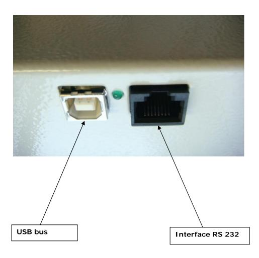
The interfaces for the digital data transfer are located on the underside of the ergometer.
